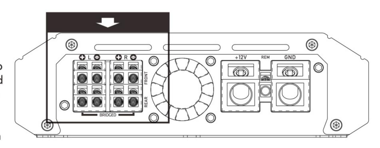
If the wires ever come in contact with each other the amplifier will go into protection.
