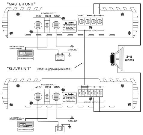
Using a dual amplifier configuration, the MASTER amplifier has total control over the SLAVE amplifier. When using dual amplifier to operate subwoofer, the positive terminal of the subwoofer's voice coil must be connected to the positive terminal of the MASTER Amplifier and the negative terminal of the subwoofer's voice coil must be connected to positive terminal of the SLAVE Amplifier.
