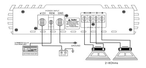
The positive and negative terminal of the subwoofer's voice coil are connected to the positive and negative terminal of the Amplifier.
